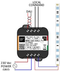
MINI-1AC-DALI has 1 output channel that can be driven independently (e.g. for AC modules).
