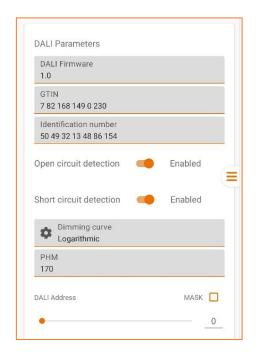
**DALI Firmware:** Identifies the DALI firmware version currently loaded on the device (non-editable field).
