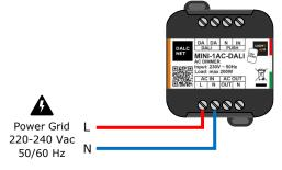
Figure 6: Power connection diagram
