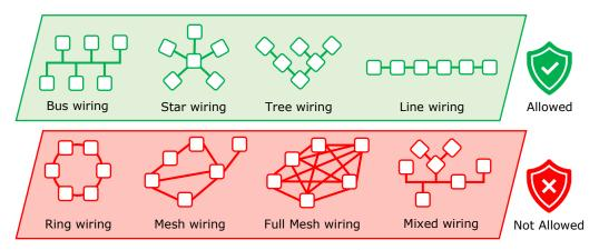
Figure 5: DALI Wiring Topologies
