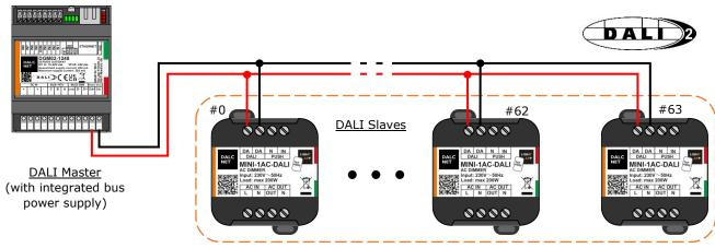
Figure 4: Remote Control Connection, Bus-wiring
