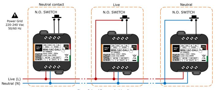
Figure 3: Local Command wiring diagram
