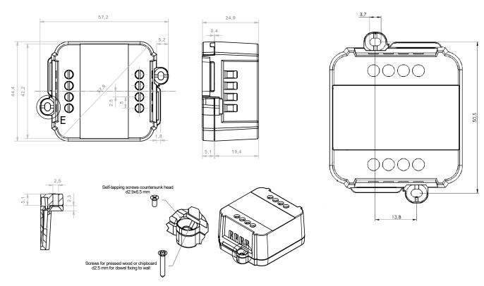
Figure 9: Mechanical dimensions
