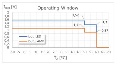
Figure 7: Temperature Operating Window
