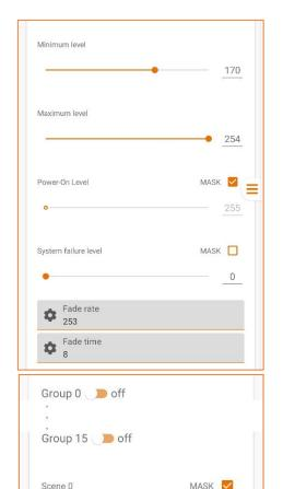
**Minimum Level:** sets the minimum level of light intensity that can be reached by remote control (default value = 1).
